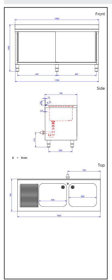
Drain: Drainer position: Left **Key Information:** Cabinet width: 1745 mm Cabinet depth: 645 mm Cabinet height: 380 mm 1800 mm External dimensions, Width: External dimensions, Depth: 700 mm External dimensions, Height: 1000 mm Upstand Dimensions, Height: 100 mm Upstand Dimensions, Depth: 13 mm Upstand Dimensions, Radius: R=10 **Bowls number Bowl dimensions** 600x500xH300 Number and type of doors: 2 Sliding Worktop thickness: 50 mm Net weight: 70 kg
